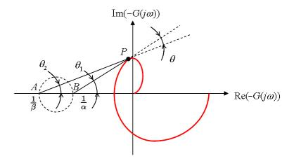
Since  $G_T(s) = G(s)[1 - \beta(-G(s))]^{-1}$  has to be Hurwitz for the result to hold, it implies that  $-G(j\omega)$  needs to encircle  $(1/\beta, 0j)$  or disk  $D(-\beta, -\alpha)$  (since  $-G(j\omega)$  does not enter the disk) counter-clockwise a number of times equal to the number of unstable poles (ORHP) of G(s).
